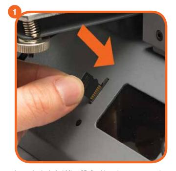
Insert the included MicroSD Card into the memory card slot next to the LCD screen with the label facing to the left as shown
