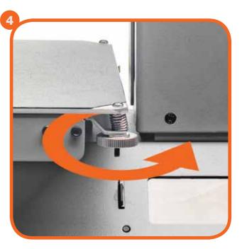
On each corner, turn the corresponding thumbwheel until you can just slide the levelling card or a piece of copy paper between the extruder and print bed with slight friction, about 0.1mm
