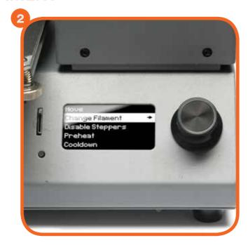
Push the dial button to access the Main Menu and navigate to **Quick Settings + Change Filament + Add Filament**. The extruder will automatically raise and preheat
