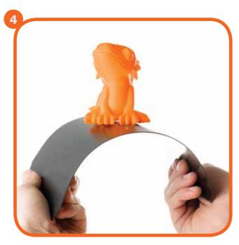
Once the print is complete, turn off your 3D Printer and wait for the extruder to cool. After removing the magnetic print mat from the printer base, slowly and gently bend the sides of the mat down to raise the center of the mat and lift the printed object
