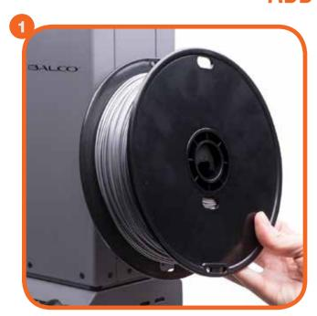
Place your roll of filament on the filament spool holder
